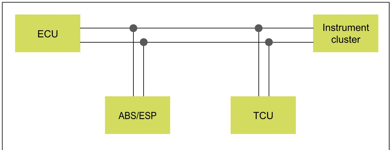
The TCU transmits the following signals via the CAN bus.
